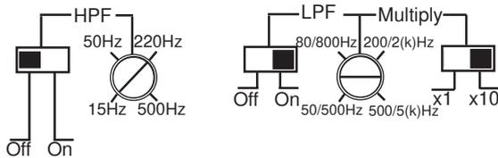
We want a crossover point of 4 kHz between tweeter and midrange. If you for some reason want to limit the low bass reproduction switch on the HPF-filter. The typical setting is then around 60 – 80 Hz. Switch the LPF-filter switch to ON and the Multiply switch to x10 position. Now you can adjust the filter setting from 500 Hz to 5 kHz. Adjust the setting to 4 kHz.
