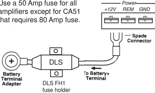
Connect the battery cable by a crimp fork terminal (spade) to the +12 Volt on the amplifier. If you use a AWG 8 = 10 mm<sup>2</sup> or thinner cable, you can do without the crimp terminal and put the cable right into the connector. Be sure to use a rubber grommet or a plastic insulating tube where the cable passes the firewall or other places when it can easily be jammed. Use wire ties to secure to existing cables in the engine compartment.
