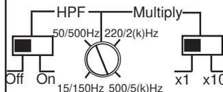
With the HPF-filter in OFF position the amplifier allows the speakers to play fullrange. If you for some reason want to limit the low bass reproduction switch on the HPF-filter. The typical setting is then around 60 – 80 Hz.
