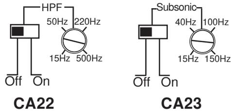
The **HPF** ( high pass filter ) blocks very low frequencies from reaching the speakers. It is mostly used at say 60 Hz to protect small speakers ( like 6 inch and smaller ) from deep bass. It can also be used as subsonic filter to take away the very deepest frequencies from a bass box. The typical setting is then around 25 – 40 Hz. CA23 has a high pass filter designed as a subsonic filter variable from 15 Hz to 150 Hz.
