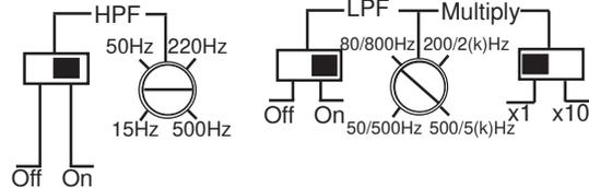
The subwoofer should be connected to channel A/ B in bridge mode. The Grand Bass mode can now be used for the subwoofer. Set the HPF-filter switch to ON-position. Adjust the filter setting to 25-40 Hz. Set the LPF-filter switch to ON-position and the Multiply switch to x1. Adjust the frequency setting to 70-90 Hz.
