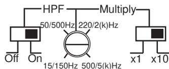
Channel C/D are used for tweeters and must be set to play from 4 kHz and up. The HPF-filter switch must be ON and the multiply switch in x 10 position. Now you can adjust the filter setting from 150Hz to 5 kHz. Adjust the setting to 4 kHz.
