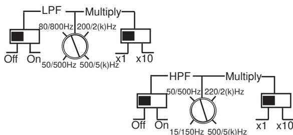
Channel A/B is equipped very much like the CA22 and CA23, however the LPF has a multiplier. Thus the frequency range of the LPF can be varied from 50 Hz – 500 Hz in the x1 position or 500 Hz – 5 kHz in the x10 position. This way we can use this amplifier to feed a 2-way system, where the midbasses are feed from 80 Hz – 4 kHz.
