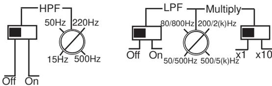
With the HPF-filter in OFF position the amplifier allows the speakers to play fullrange. If you for some reason want to limit the low bass reproduction switch on the HPF-filter. The typical setting is then around 60 – 80 Hz. The LPF-filter switch should be in OFF-position
