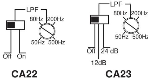
The **LPF** ( low pass filter ) mostly used for subwoofers. It will allow low frequencies only and blocks higher frequencies.
