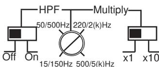
With the HPF-filter in OFF position the amplifier allows the speakers to play fullrange. If you for some reason want to limit the low bass reproduction switch on the HPF-filter. The typical setting is then around 25 – 40 Hz.
