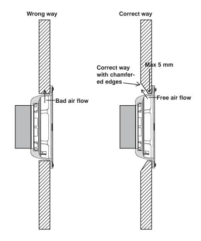
It is very important that the baffle is stable, but it is just as important that it is shaped in a way that allows the driver to "breath" backwards, otherwise there will be a lack in the drivers bass reproduction.
