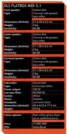
DLS's Midi range of Flatbox speakers continues the company's wall-mounted concept. It entails relatively compact creations which can fit just about anywhere. It is simplest to mount the speakers using the integrated keyholes. The speakers are then distanced from the wall through rubber pads which also ensure that there are no rattles and that cabinets and walls are not scratched. The cabinet is bass reflex with an upwardly directed slot on the cabinets' short side.
