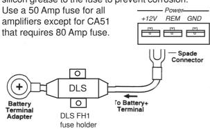
Connect the battery cable by a crimp fork terminal ( spade ) to the +12 Volt on the amplifier. If you use a AWG  $8 = 10 \text{ mm}^2$  or thinner cable, you can do without the crimp terminal and put the cable right into the connector.
