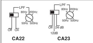
The LPF (low pass filter) mostly used for subwoofers. It will allow low frequencies only and blocks higher frequencies.
