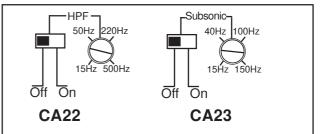
The **HPF** (high pass filter) blocks very low frequencies from reaching the speakers. It is mostly used at say 60 Hz to protect small speakers (like 6 inch and smaller ) from deep bass. It can also be used as subsonic filter to take away the very deepest frequencies from a bass box. The typical setting is then around 25-40 Hz. CA23 has a high pass filter designed as a subsonic filter variable from 15 Hz to 150 Hz.
