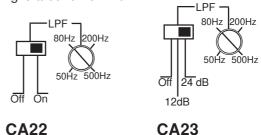
The LPF will allow low frequencies only and blocks higher frequencies. A typical setting is 70-90 Hz. In the CA23 amplifier you can select between two different slopes, 12 dB/ octave or 24 dB/ octave. Choose the slope and the setting that sounds best in your car.
