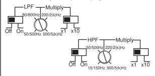
Channel A/B is equipped very much like the CA22 and CA23, however the LPF has a multiplier. Thus the frequency range of the LPF can be varied from 50~Hz-500~Hz in the x1 position or 500~Hz-5~kHz in the x10 position. This way we can use this amplifier to feed a 2-way system, where the midbasses are feed from 80~Hz-4~kHz.
