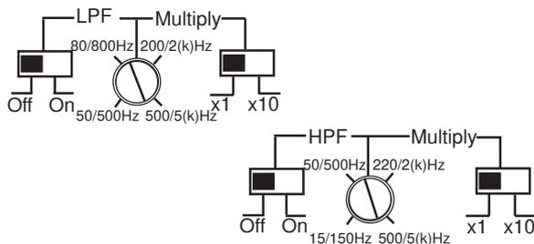
Channel A/B is equipped very much like the CA22 and CA23, however the LPF has a multiplier. Thus the frequency range of the LPF can be varied from 50 Hz – 500 Hz in the x1 position or 500 Hz – 5 kHz in the x10 position. This way we can use this amplifier to feed a 2-way system, where the midbasses are feed from 80 Hz – 4 kHz.
