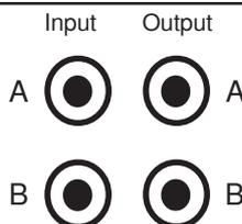
Use RCA Outputs to connect additional amplifiers (not available on PA31 & PA51).
