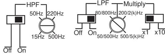
The subwoofer should be connected to channel A/ B in bridge mode. The Grand Bass mode can now be used for the subwoofer. Set the HPF-filter switch to ON-position. Adjust the filter setting to 25-40 Hz. Set the LPF-filter switch to ON-position and the Multiply switch to x1. Adjust the frequency setting to 70-90 Hz.
