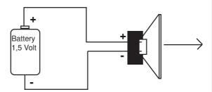
**NOTE!** Tweeters can not be tested this way, double check the connections instead.
