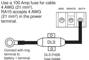
Connect the battery cable from the fuse holder to the +12 Volt terminal on the amplifier.
