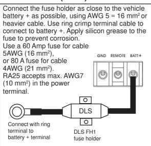
Connect the battery cable from the fuse holder to the +12 Volt terminal on the amplifier.
