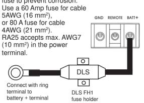
Connect the battery cable from the fuse holder to the +12 Volt terminal on the amplifier.
