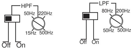
The **MRA31** is a three channel amplifier. It has a variable high pass filter, 50-150 Hz, for channel A/B. The C channel is for subwoofers and has a subsonic filter, a variable low pass filter, 50-120 Hz, and a phase control variable from 0 - 180 degrees. The subsonic filter can be switched IN-OUT and has a fixed frequency of 25 Hz.
