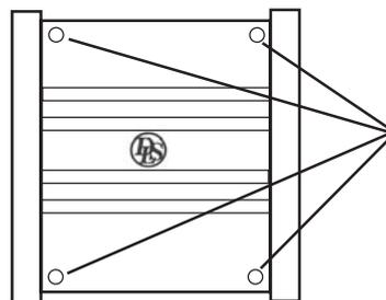
Remove these screws using a 3 mm hex. key for removal of side flange. Remount after attaching the amplifier and connection of the speaker and power cables.
