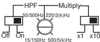
Channel C/D are used for tweeters and must be set to play from 4 kHz and up. The HPF-filter switch must be ON and the multiply switch in x 10 position. Now you can adjust the filter setting from 150Hz to 5 kHz. Adjust the setting to 4 kHz.
