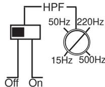
The HPF filter is here used as subsonic filter to take away the very deepest frequencies. The typical setting is around 25 – 40 Hz.
