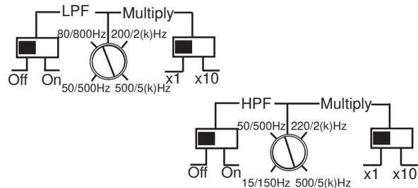
Channel A/B is equipped very much like the MRA22, however the LPF has a multiplier. Thus the frequency range of the LPF can be varied from 50 Hz – 500 Hz in the x1 position or 500 Hz – 5 kHz in the x10 position. This way we can use this amplifier to feed a 2-way system, where the midbasses are fed from 80 Hz – 4 kHz.
