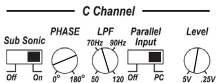
The **MRA41** is a four channel amplifier. It is mostly used with a front system connected to channels C/D and a subwoofer connected to channel A/B. You will find speaker wiring and filter setting example on page 9. Please observe the proper settings of the channel A/B LPF multiplier switch and of the channel C/D HPF multiplier switch.
