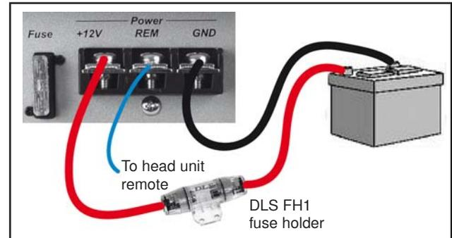
Connect the battery cable by a crimp fork terminal (spade) to the +12 Volt on the amplifier. Do likewise with the negative cable. If you use a AWG 8 = 10 mm<sup>2</sup> or thinner cable, you can do without the crimp terminal and put the cable right into the connector. Be sure to use a rubber grommet or a plastic insulating tube where the cable passes places when it can easily be jammed. Use wire ties to secure to existing cables.
