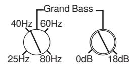
**Grand Bass** is used to increase the bass volume at an interval of bass frequencies. You can select the center frequency between 25Hz and 80 Hz and the amplification between 0 dB ( no amplification ) and 18 dB ( full amplification ).
