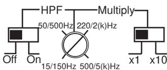
With the HPF-filter in OFF position the amplifier allows the speakers to play fullrange. If you for some reason want to limit the low bass reproduction switch on the HPF-filter. The typical setting is then around 60 – 80 Hz.
