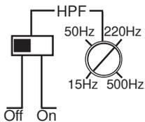
With the HPF-filter in OFF position the amplifier allows the speakers to play fullrange. If you for some reason want to limit the low bass reproduction switch on the HPF-filter. The typical setting is then 60 – 80 Hz.
