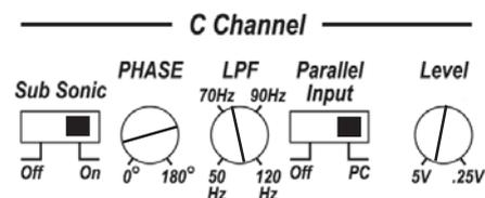
The subsonic filter takes away the very deepest frequencies. Turn on the subsonic filter if you want to remove these frequencies.
