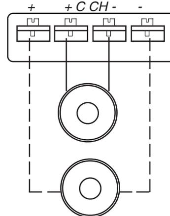
A single 2 ohm subwoofer can also be connected.
