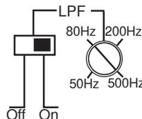
The LPF will allow low frequencies only and blocks higher frequencies. A typical setting is 70 – 90 Hz.
