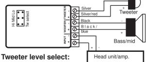
Select tweeter level by moving the jumper inside the filter box between high, mid or low. Make your own tests for best result.
