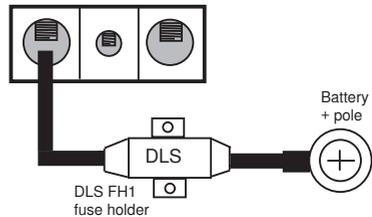
Be sure to use a rubber grommet or a plastic insulating tube where the cable passes the firewall or other places where it can be easily jammed. Use wire ties to secure to existing cables in the engine compartment.
