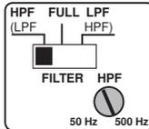
Set the switch in position **HPF** to activate the filter. Test which setting sounds best. The filter can be set at **FULL** position if you want to run the amplifier in full range mode without limiting the frequency range.
