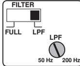
Set the switch in **LPF** position to activate the filter. Set the switch in **FULL** position if you want to run the amplifier in full range mode.
