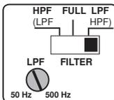
Set the switch in **LPF** position to activate the filter. Set the switch in **FULL** position if you want to run the amplifier in full range mode.
