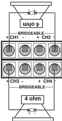
One 4 ohm subwoofer connected to channels 1 / 2 and one 4 ohm subwoofer to channels 3 / 4.
