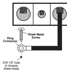
A cable up to AWG 4 ( 21 sq mm) fits the amplifier ground (GND) terminal
