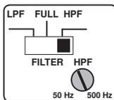
Set the switch in position **HPF** to activate the filter. Adjust with the **HPF control** after your own taste, a normal setting is 50 - 70 Hz.
