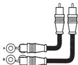
**XM40** has dual inputs **CH1 / CH2 / CH3 / CH4** Depending on your chosen configuration you can use either two separate RCA cables, or a single RCA cable together with an Y-split to connect both inputs.
