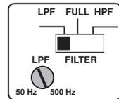
Set the switch to **LPF** position to activate the filter. Use this position when connected to a subwoofer.
