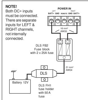
Connect the fuse holder as close to the vehicle battery + as possible, using AWG 4 = 21 mm<sup>2</sup> or heavier cable. Use ring crimp terminal cable to connect to battery +. Apply silicon grease to the fuse to prevent corrosion. Connect to amplifiers + inputs via a Fuse block. The amp terminals accept 16 mm<sup>2</sup> (AWG5) cable size
